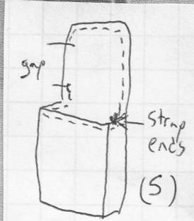
(5) place lining inside reticule, right sides together. Ensure strap ends protrude above seam. Sew 0.25" seam along top edges, leaving a gap as shown.
